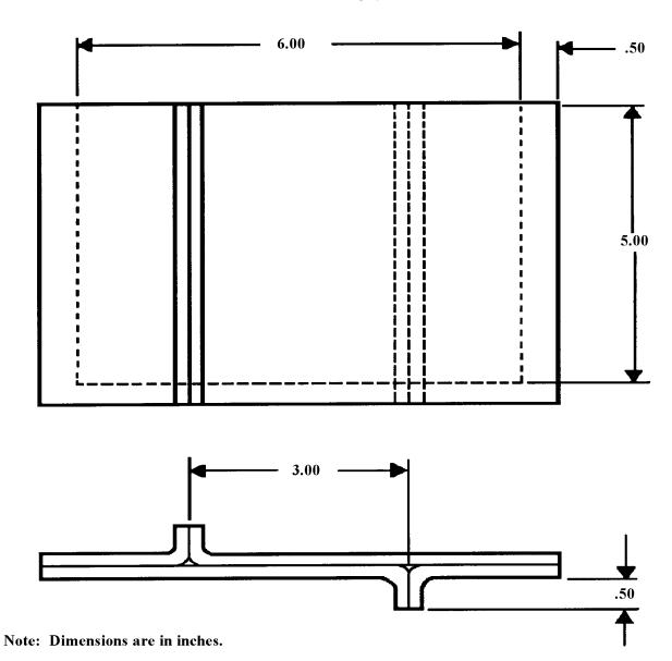
FIGURE 2. Pouch for seam fabrication test.
